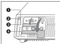
Open the cover to use the INPUT A or Video input connectors.
