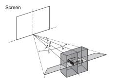
**a:** Tilting angle of the projector in the "V Keystone" adjustment area **b:** "Side Shot" (H Keystone adjustment) area
