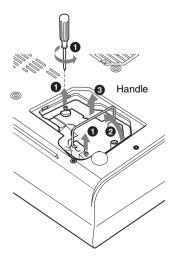
**5** Insert the new lamp all the way in until it is securely in place (1). Tighten the two screws (2). Fold down the handle to replace it (3).
