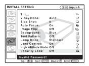
**4** Turn the main power off and disconnect the AC power cord. The security lock is set to on, then it becomes effective. The screen used for entering the password is displayed when the power is turned on the next time.
