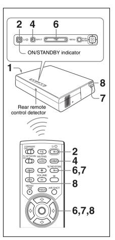
Plug the AC power cord into a wall outlet, then connect all equipment. The ON/STANDBY indicator lights in red and the projector goes into standby mode.
