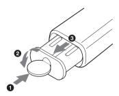
Open the cover (2) with a coin (1) and remove the battery case (3). Install the two size AAA (R03) batteries with the correct polarity.
